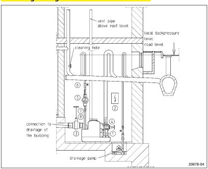
All types have DN 80 / PN 10 connecting flange, however with pipe socket DN 100. For this reason, a non-return valve for the pressure pipe need to be chosen for DN 80 only in case of direct erection. The downstream pressure pipe is connected to DN 100 by an elastic connection.
