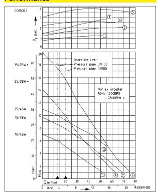
We reserve the right to change specifications without notice Pump performance is subject to ISO 9906 tolerances The minimum flow velocity in the pressure piping must be 0.7 m/s according to EN 12056. This data is represented in the performance curve as a limit of application.
