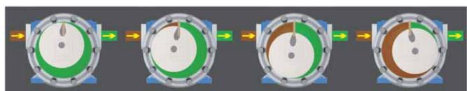
The hollow disc is eccentrically mounted in the rotor shaft and turns around the suction and discharge cameras separator vane. In this way the piston is obliged to follow the trajectory around the vane and externally to the pump head, where it is pushed via an elastic device internally inserted. A silent and reliable pumping is achieved, without vortexes nor liquid breakages, for viscous fluids even above 10000 cst.
