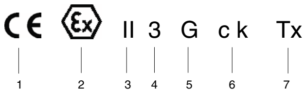
Fig. 15 Explosion protection labeling on the pump (equipment group II, category 3)
