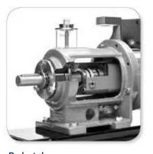
**Pedestal** over-sized bearing, regulation of rotor and drip tray integrated in one cast.
