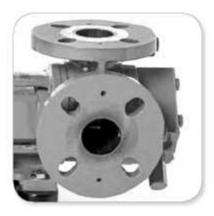
**DIN or ANSI flanged ports** from DN40 to DN250, with through-holes to facilitate the installation. ¼" threaded holes for vacuum/pressure gauge.
