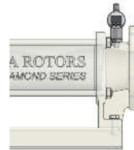
Overpressure valve flanged or with threaded couplings GAS BSP. This part discharges the overpressure that generates in delivery to the pump and transfers the flow outwards. Usable up to 40 bar. Particularly strong and suitable for heavy use with viscous fluids or containing abrasive solids. It is used in the bypass to re-integrate the fluid in the body of the pump.
