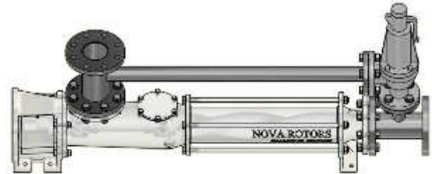
Separate funnel very useful to reduce rotor maintenance times if the pump is big or has complex system installation. It enables dismantling of the rotor without disconnecting the pump from the system and without removing the body of the pump.
