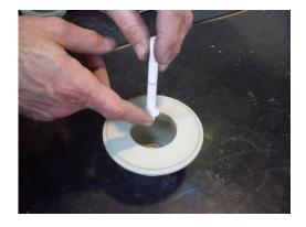
8) Pull out the shaft and the rear ring, check status and replace if necessary.
