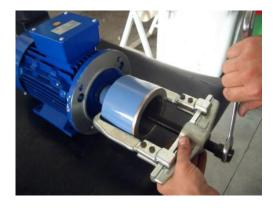
10) Using an extractor pull-out the external magnet from motor shaft.
