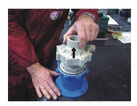
6) Pull out the internal assembly from the bracket. Check status of all internal parts and replace it if necessary.
