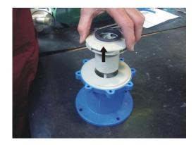
7) Pull out the rear casing with the shaft.
