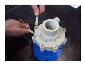
5) Pull out the pump casing and then verify the status of the O-ring and pump casing thrust bearing.
