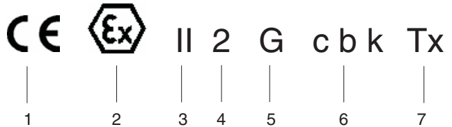
Fig. 14 Explosion protection labeling on the pump (equipment group II, category 2)
