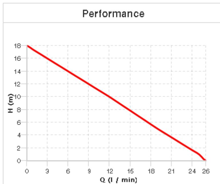
Characteristics referring to operation with water at 20°C
