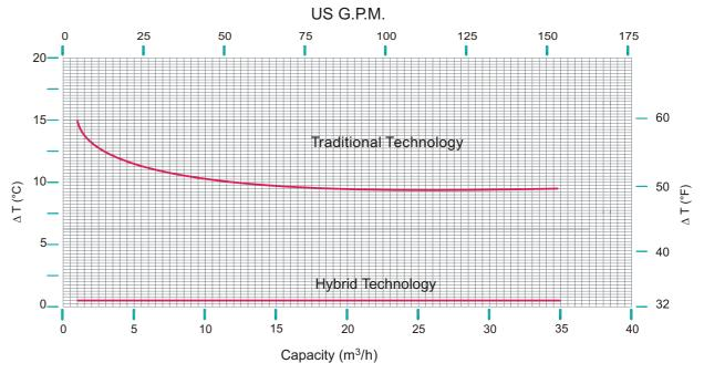
Hybrid technology reduces greatly heat generation in the rear casing region. This beneft is particularly important when pumping low boiling liquids.
